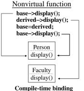
The function to be called is determined by the type of the pointer during compilation.
