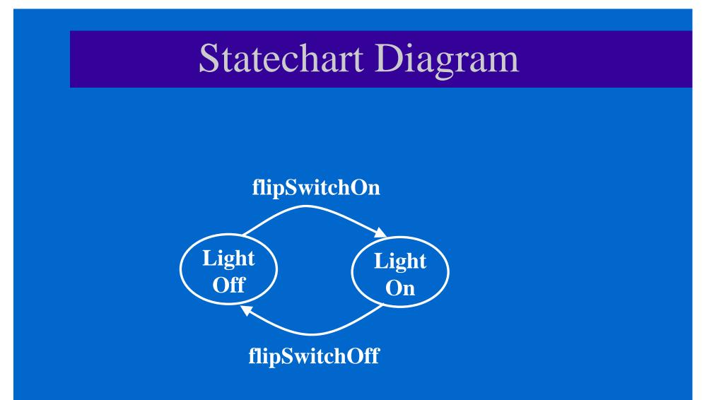
**Transitions between states of an object** (Extension of Finite State Machine (FSM) model)
